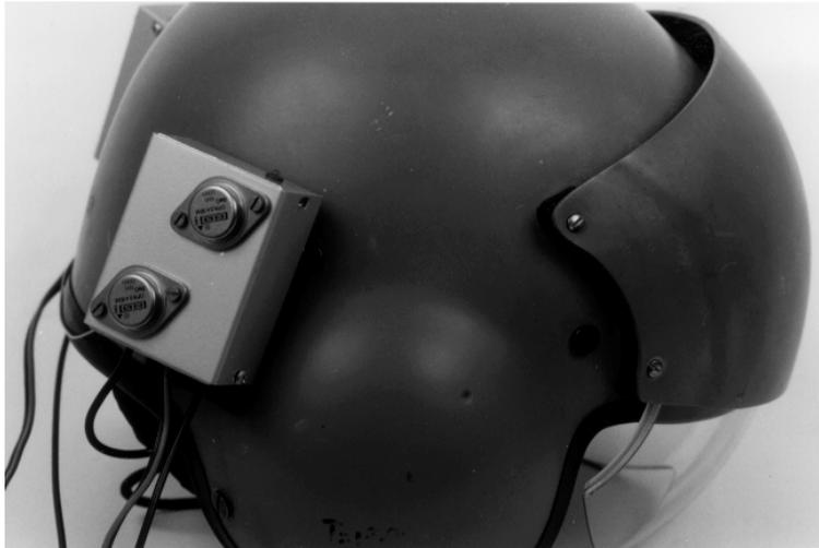
Figure 2. Helmet with w-CEP transmitters
