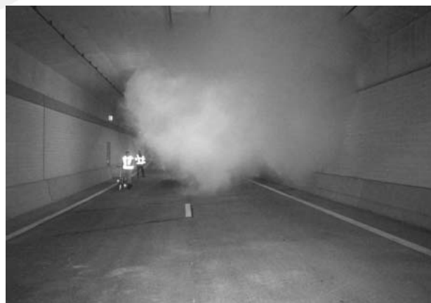
Fig. 3. Tunnel interior while smoke is being produced in preparation for experiment.
