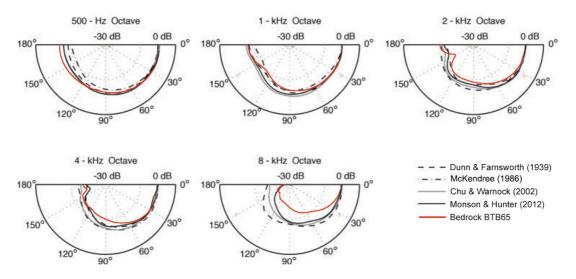
Figure 8. Directivity of the Bedrock BTB65 in the horizontal plane (red curve), compared with the directivity of human speech according to 4 different studies (after [6]). Data for lower octave bands have been omitted, since the BTB65 as well as human talkers show near-perfect omnidirectional behaviour.
