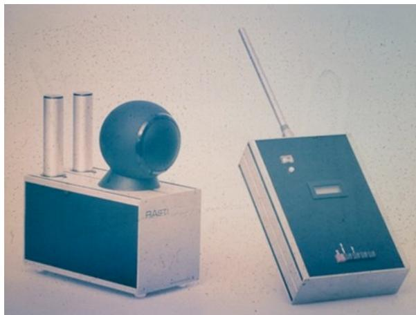
Figure 2. First implementation of RASTI in hardware (1980).
