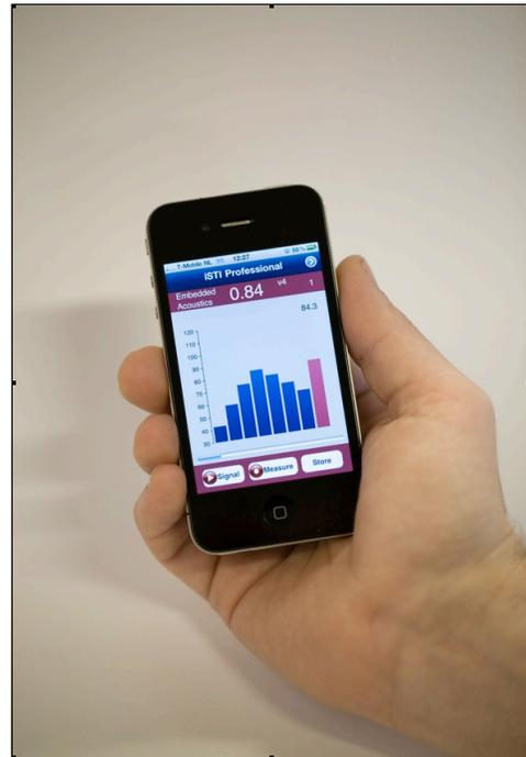
Figure 4. iPhone app for performing 4<sup>th</sup> edition-compliant STIPA measurements (2011)
