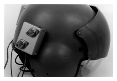
Figure 2. Helmet with w-CEP transmitters
