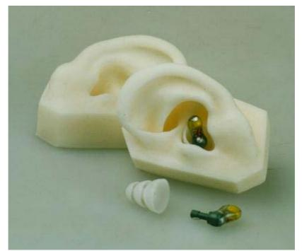
Figure 4. Wireless Communications Earplug receivers (in an artificial ear and separately).
