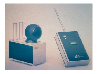
Figure 2. First implementation of RASTI in hardware (1980).
